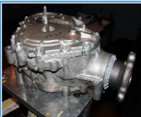
Figure 4 - Aluminum 4-wheel-drive Power Transfer Unit assembled with TAPTITE 2000® screws
