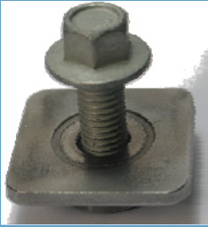
Figure 1 - Pierce-and-Clinch Nut assembled in HSLA thin-sheet steel
